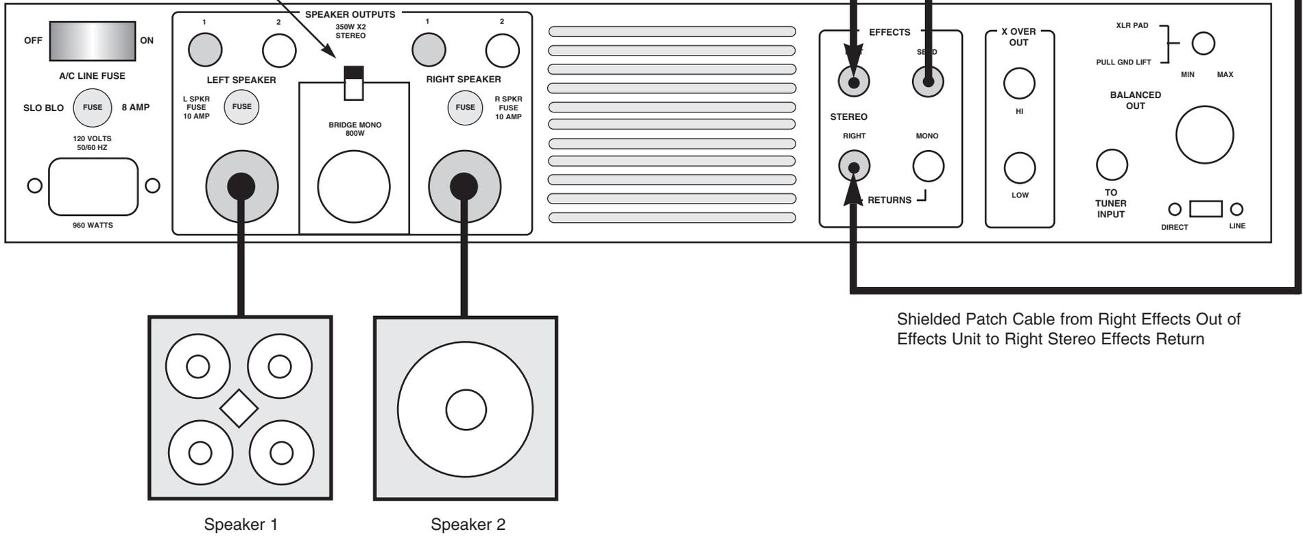
Shielded Patch Cable from Right Effects Out of Effects Unit to Right Stereo Effects Return
