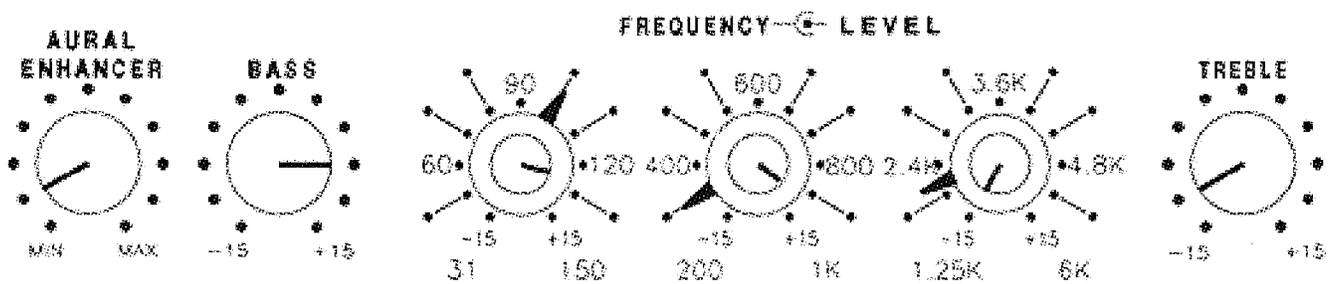
panel. For example, if the Frequency is set at mid-position or 500Hz, all frequencies BELOW 500 Hz will appear at the LOW output jack. All frequencies ABOVE 500Hz will be present at the HI output jack.
